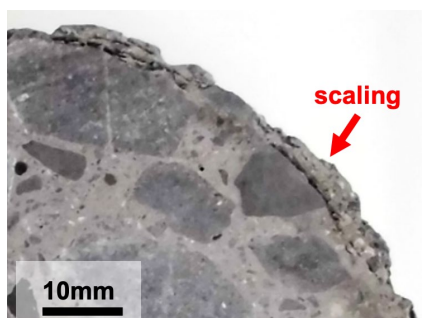
FIGURE 4: Concrete specimen immersed in a paste of incineration fly ash (No. 5).
