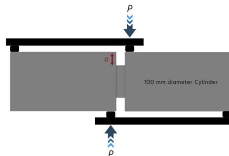
FIGURE 2. Shear setup for concrete specimens (26).
