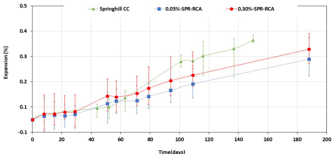
FIGURE 3. Expansion as a function of time for concrete mixtures (6).
