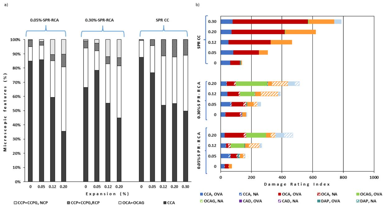
FIGURE 5. a) Percentage of distress features and b) DRI chart in CC and RCA concrete (6).
