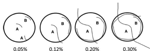
FIGURE 1. A qualitative model of crack propagation in ASR-affected CC (10).
