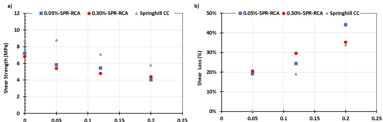
FIGURE 4. a) Direct shear strength of ASR affected specimens, and b) shear loss of ASR affected specimens at distinct expansion levels.
