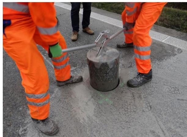
FIGURE 3. Sampling of a large (Ø 350 mm) core from a shoulder slab.
