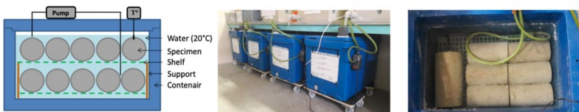
FIGURE 2. Conservation containers for DEF development.
