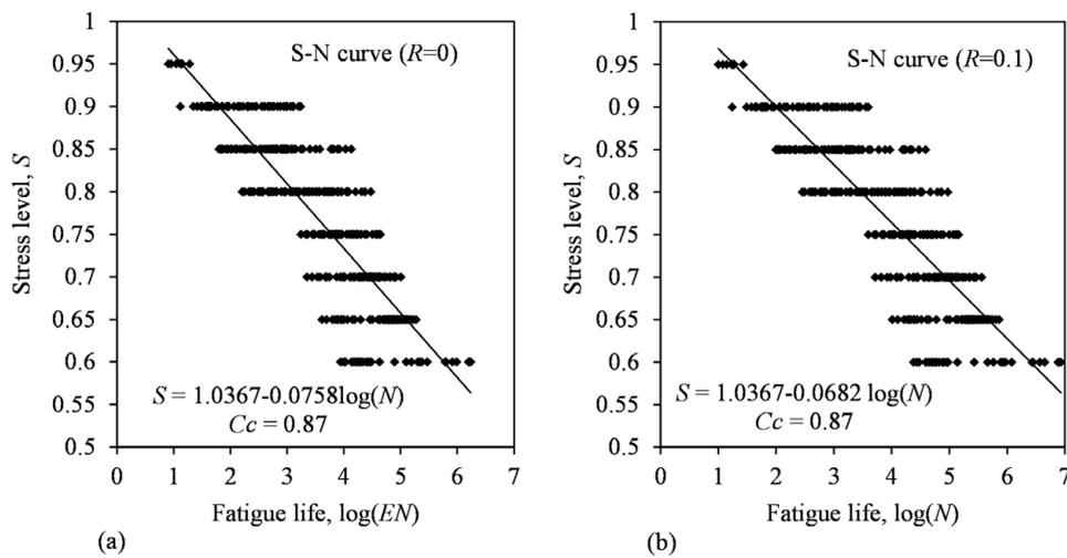
FIGURE 1. *S-N* curves (Wöhler fatigue curves) of NWC for (a)  $R = 0$  and (b)  $R = 0.1$ .
