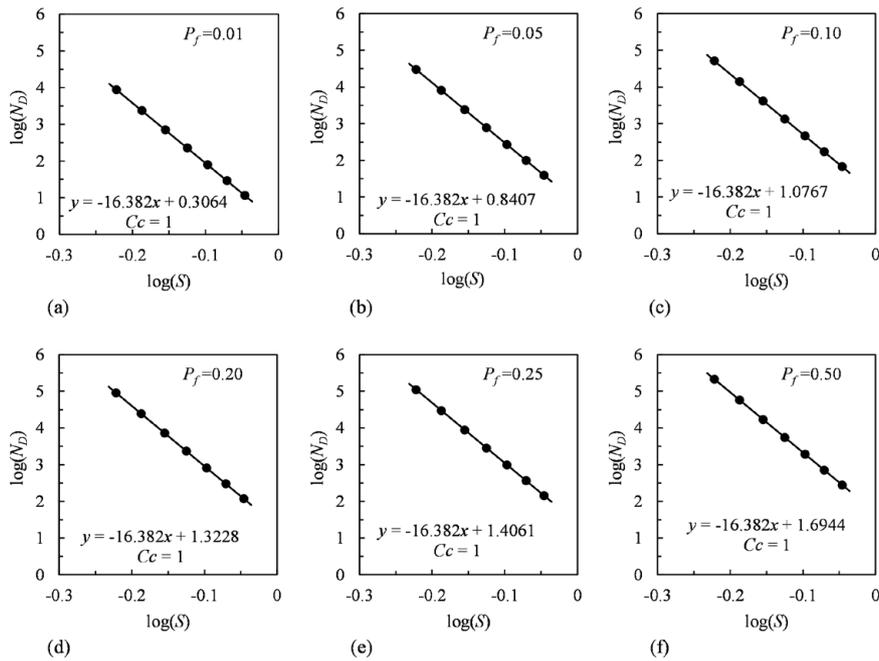
FIGURE 3.  $S$ - $N$ - $P_f$  curves for stress ratio  $R = 0$  and the failure probabilities of (a) 0.01, (b) 0.05, (c) 0.10, (d) 0.20, (e) 0.25, and (f) 0.50.
