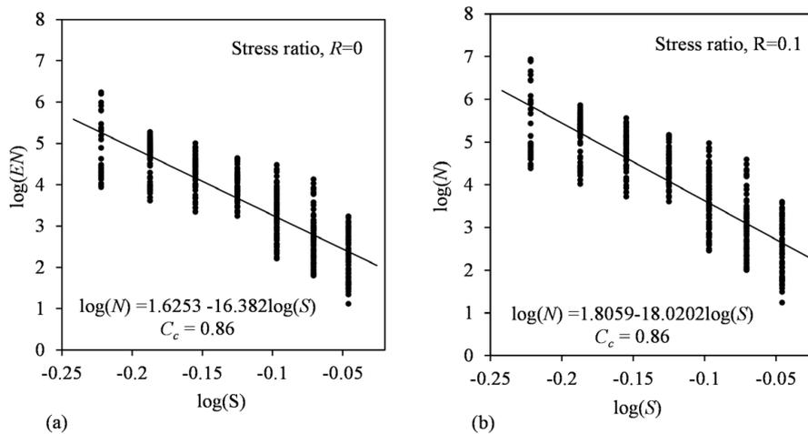
FIGURE 2. Estimating the empirical constants of *S-N* power relationships for stress ratio  $R$ : (a)  $R = 0$  and (b)  $R = 0.1$ .
