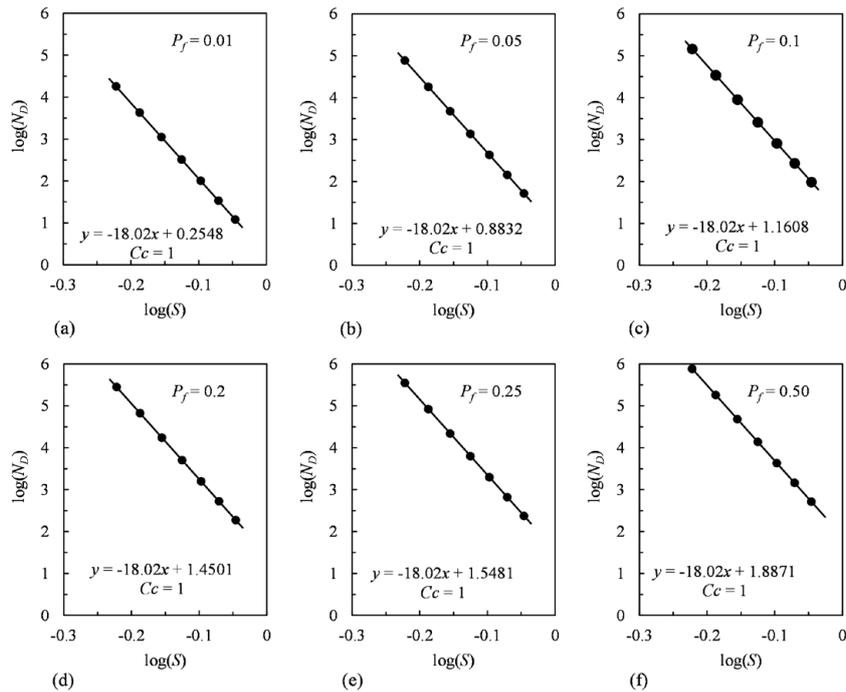
FIGURE 4.  $S$ - $N$ - $P_f$  curves for stress ratio  $R = 0.1$  and the failure probabilities of (a) 0.01, (b) 0.05, (c) 0.10, (d) 0.20, (e) 0.25, and (f) 0.50.
