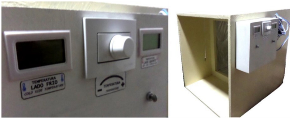
FIGURE 4. Details of the apparatus developed for the thermal chamber behavior experiment.
