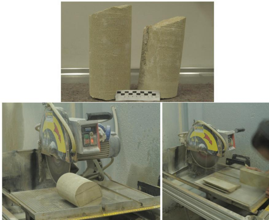
FIGURE 2. Novelda stone cores used to obtain the samples. It is shown the cut and orientation of the samples with respect to the cores.
