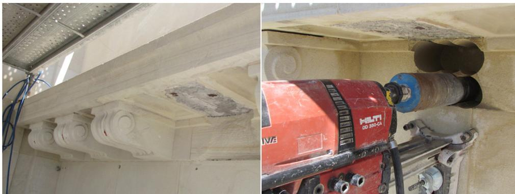
FIGURE 1. Location of the detached modillion and testification of the cores.
