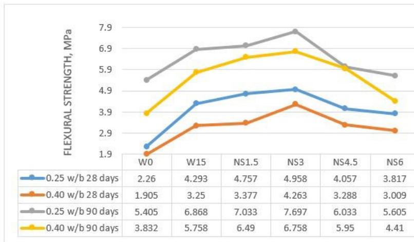
FIGURE 4. Flexural strength of paste mixes.
