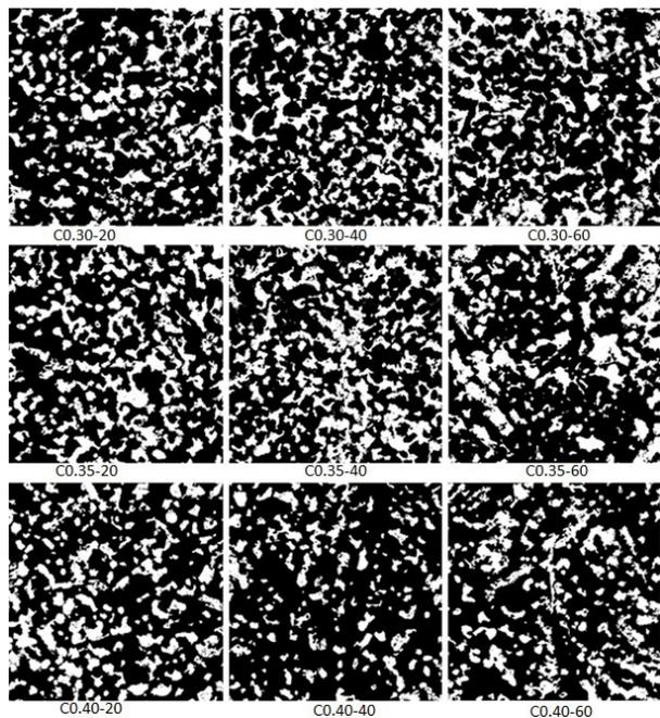
FIGURE 13. Porosity calculation based on 2D images.
