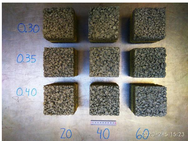
FIGURE 1. Aspect of the specimens made with different W/C ratios (horizontal label) and vibration times (vertical label).
