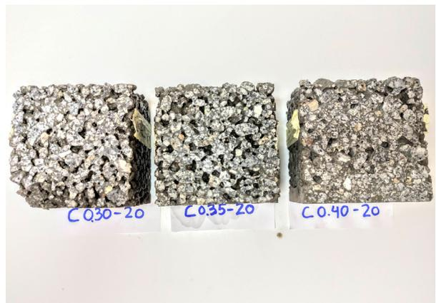
FIGURE 15. Visual observation of the porosity in the cut of the specimen section for each type of W/C mixture.
