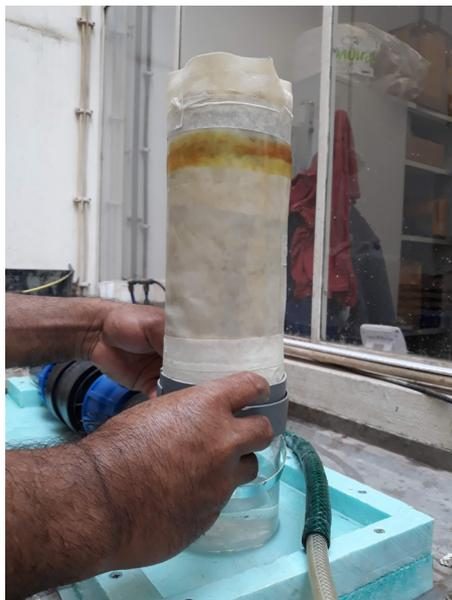
FIGURE 2. a) Schematics of the falling head permeability test apparatus and b) image of specimen preparation.
