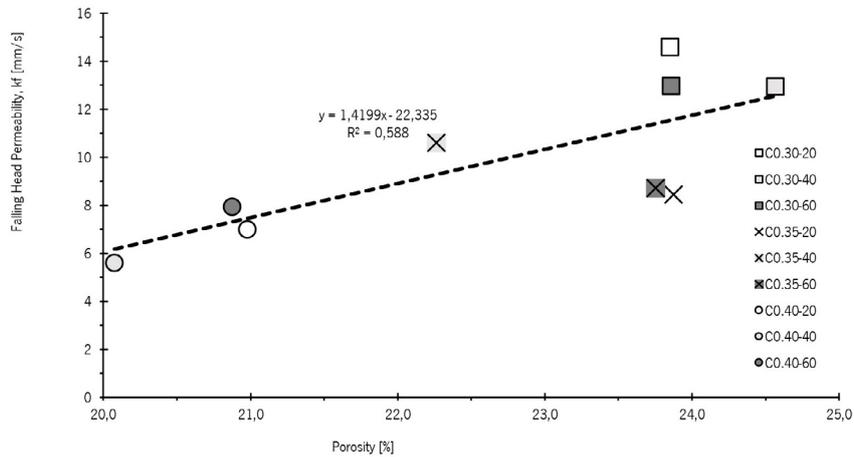
FIGURE 7. Permeability in falling head test.
