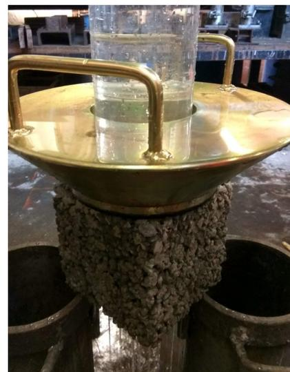
FIGURE 3. a) Schematics (32) and b) image of the permeameter used to quantify flow.
