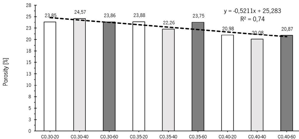
FIGURE 6. Effect of vibration and W/C ratio on porosity of Portland cement pervious concrete.
