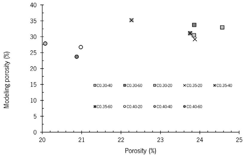
FIGURE 14. Correlation between modeling porosity and porosity.
