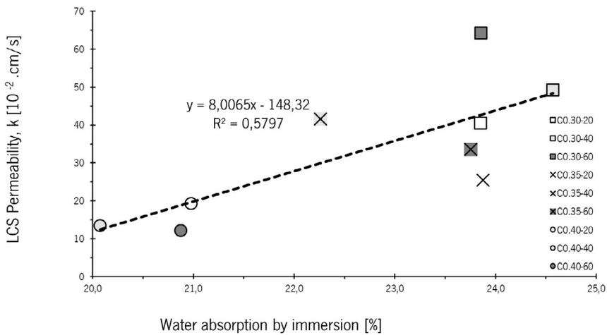
FIGURE 8. Permeability in LCS test.
