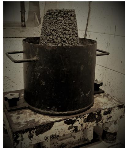
FIGURE 4. a) Slump test and b) Vee bee test.
