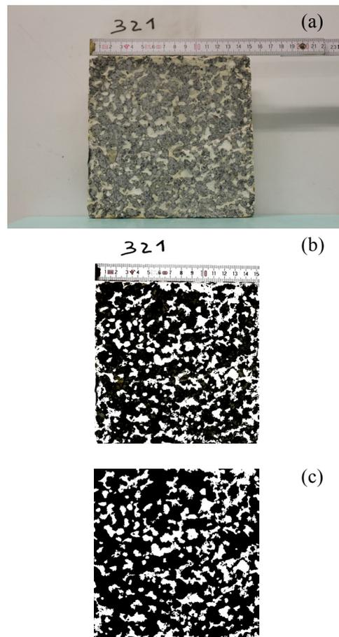
FIGURE 12. Examples of different stages of the porosity analysis procedure performed on a C0.30-20 specimen: [a] untreated image; [b] 8-bit back and white image; [c] image detail.
