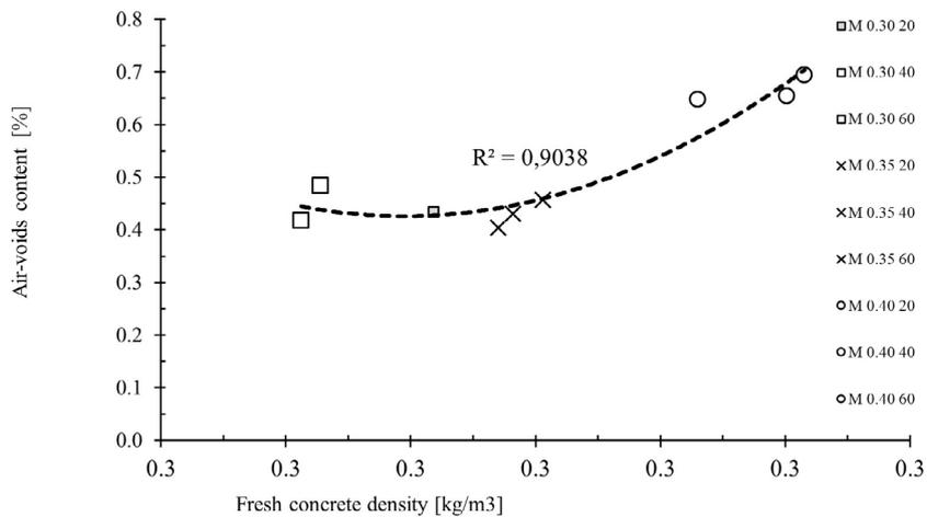
FIGURE 5. Correlation between air content and fresh concrete density.
