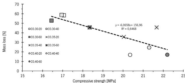
FIGURE 11. Correlation between compressive strength and mass loss by abrasion.
