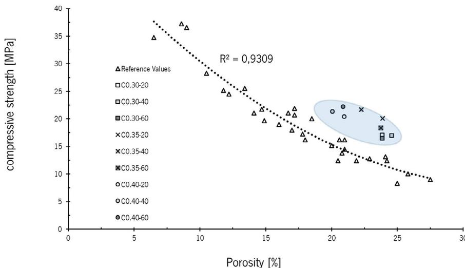
FIGURE 10. Correlation between compressive strength, porosity and reference values (39).
