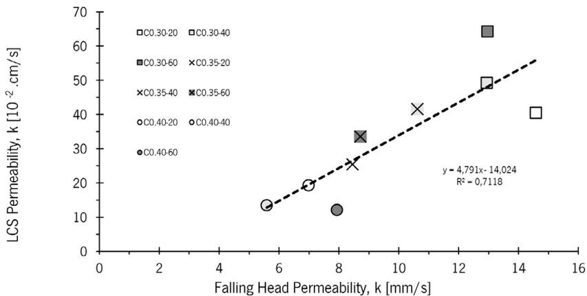
FIGURE 9. Correlation between falling head and LCS permeability.
