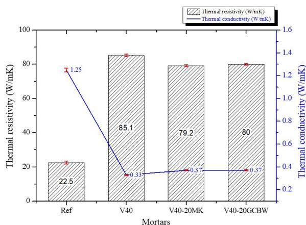
FIGURE 14. Thermal conductivity and resistivity in mortars.
