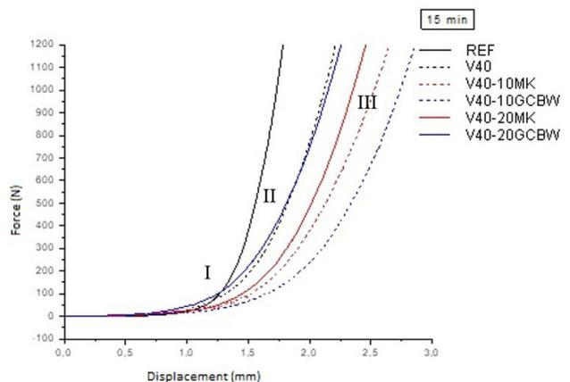
FIGURE 8. Squeeze-Flow results for the mortars after 15 minutes of mixing.
