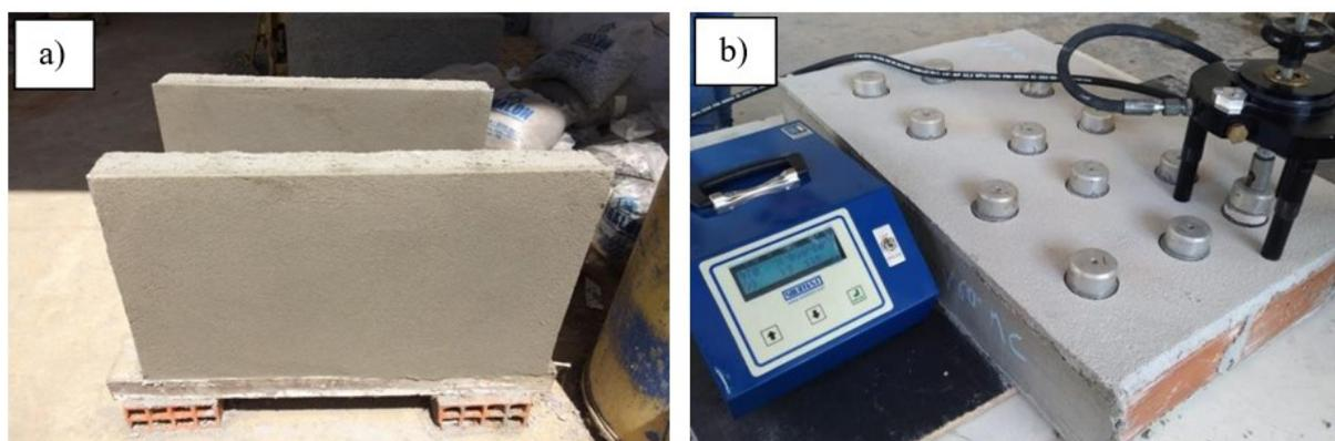
FIGURE 6. Illustration of the devices, samples, and tensile strength test a) panel made for the scratch test b) test run.
