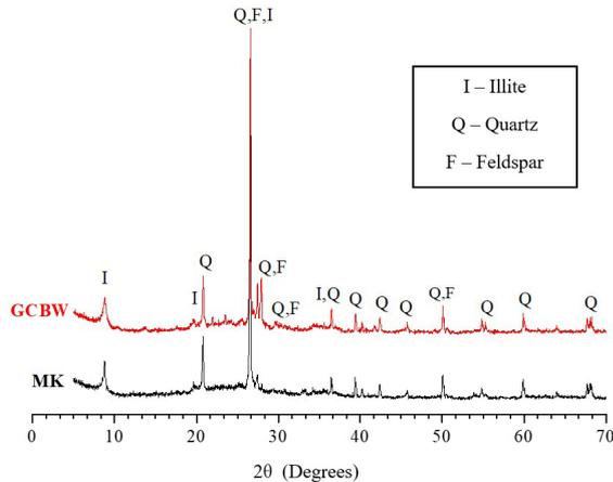
FIGURE 3. X-ray diffractogram of MK and GCBW.
