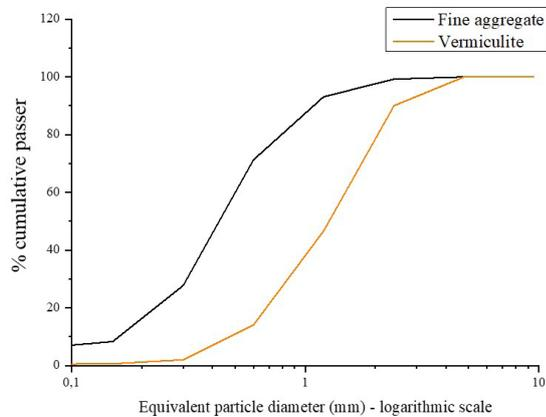
FIGURE 1. Particle size of fine aggregate and vermiculite.
