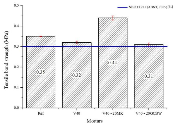
FIGURE 13. Tensile bond strength (MPa).
