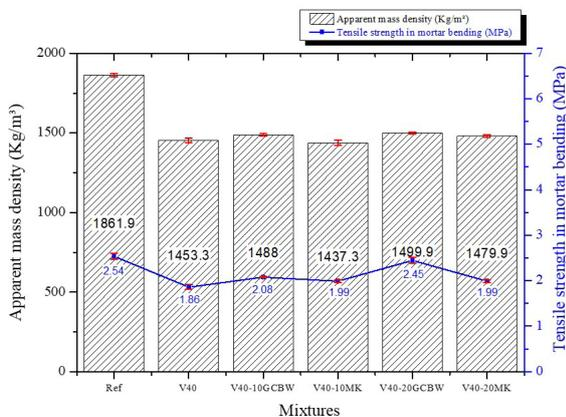
FIGURE 11. Apparent bulk density and flexural tensile strength in mortars.
