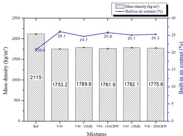
FIGURE 7. Mass density and air content incorporated in the mortars.
