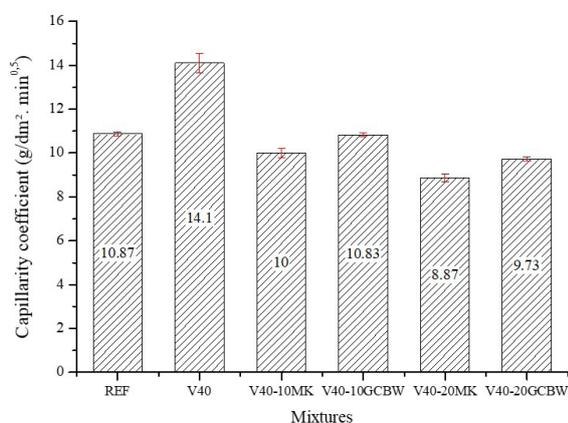
FIGURE 12. Capillarity coefficient in mortars.
