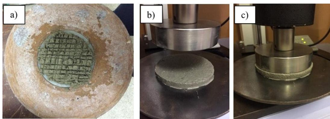
FIGURE 5. Illustration of the device and the Squeeze-Flow test a) mold used, b) sample ready for testing, c) sample being tested.
