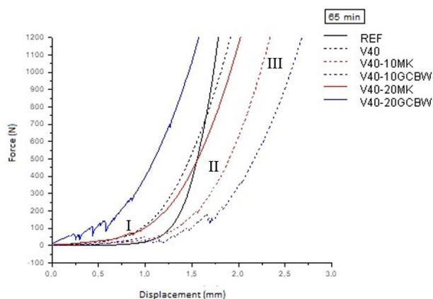
FIGURE 9. Squeeze-Flow results for the mortars after 65 minutes of mixing.
