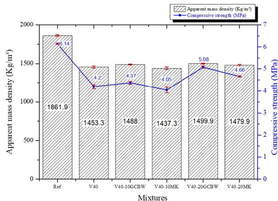
FIGURE 10. Apparent mass density and compressive strength in mortars.
