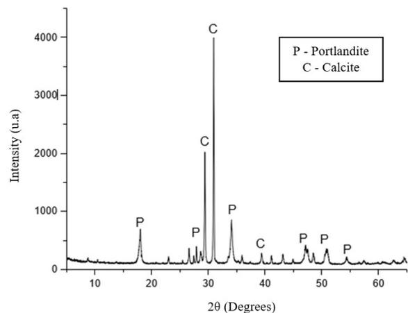
FIGURE 4. X-ray diffractogram of hydrated lime (CH - I).
