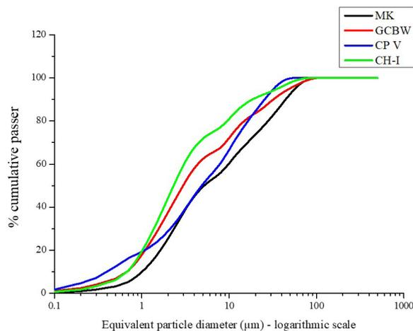
FIGURE 2. Particle size distribution curve of the fine materials.
