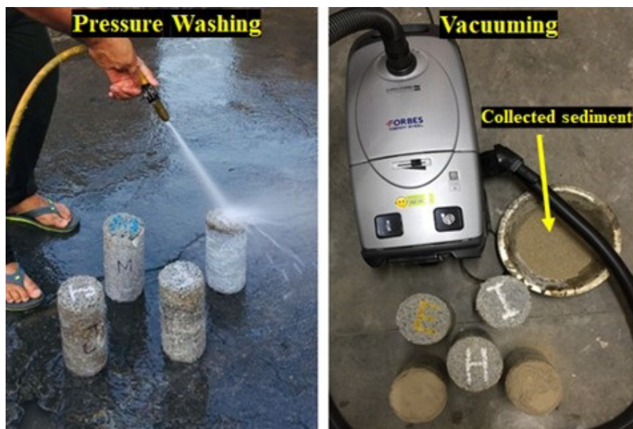
FIGURE 17. Rejuvenation of clogged specimen of pervious concrete.
