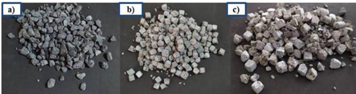
FIGURE 11. Visual appearance after crushing test (a) NA (b) SA (c) FISA.
