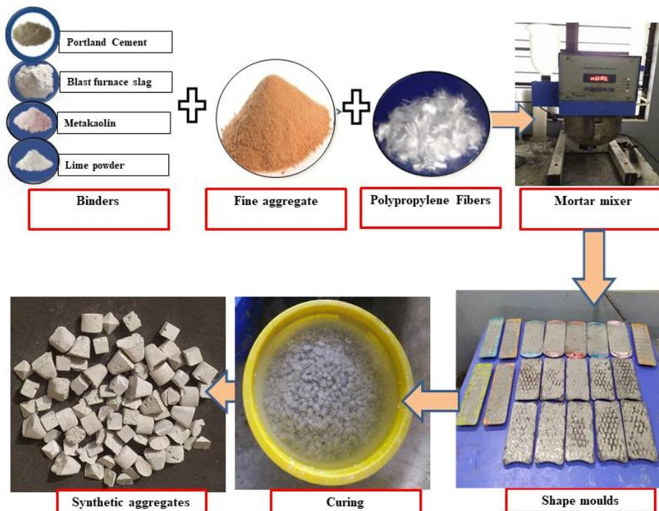
FIGURE 5. Manufacturing process of synthetic aggregates.
