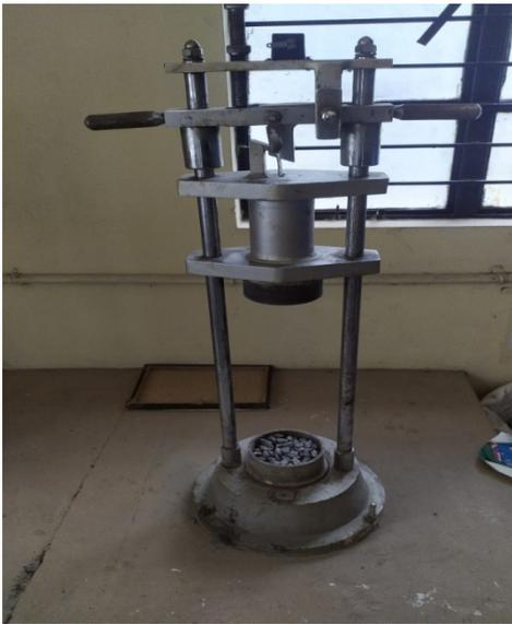
FIGURE 12. Aggregate Impact test apparatus.
