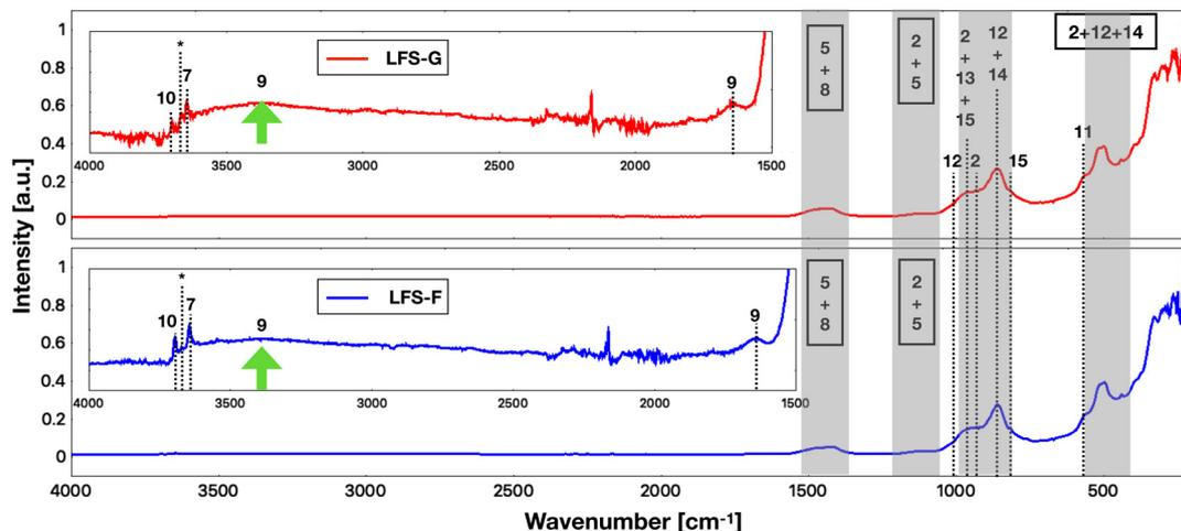
FIGURE 4. ATR-FTIR spectra of as-received LFS-G and LFS-F samples, where annotations indicate: (2)  $\beta$ - $C_2S$ ; (5) calcite; (7) portlandite; (8) periclase; (9) C-S-H gel; (10) brucite; (11) wüstite; (12) merwinite; (13) gehlenite; (14) mayenite; and (15)  $\gamma$ - $C_2S$ .
