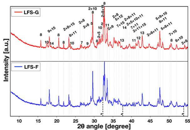
FIGURE 3. XRD diffractograms of as-received LFS-G and LFS-F samples with characteristic CaO peaks (dotted black lines), where annotations indicate: (2)  $\beta$ - $C_2S$ ; (5) calcite; (7) quartz; (8)  $\gamma$ - $C_2S$ ; (9) portlandite; (10) gehlenite; (11) merwinite; (12) wüstite; (13) periclase; (14) brucite; (15) mayenite; and (▲) free CaO.
