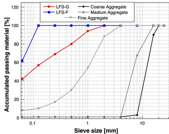
FIGURE 1. Aggregate and LFS particle size distributions.
