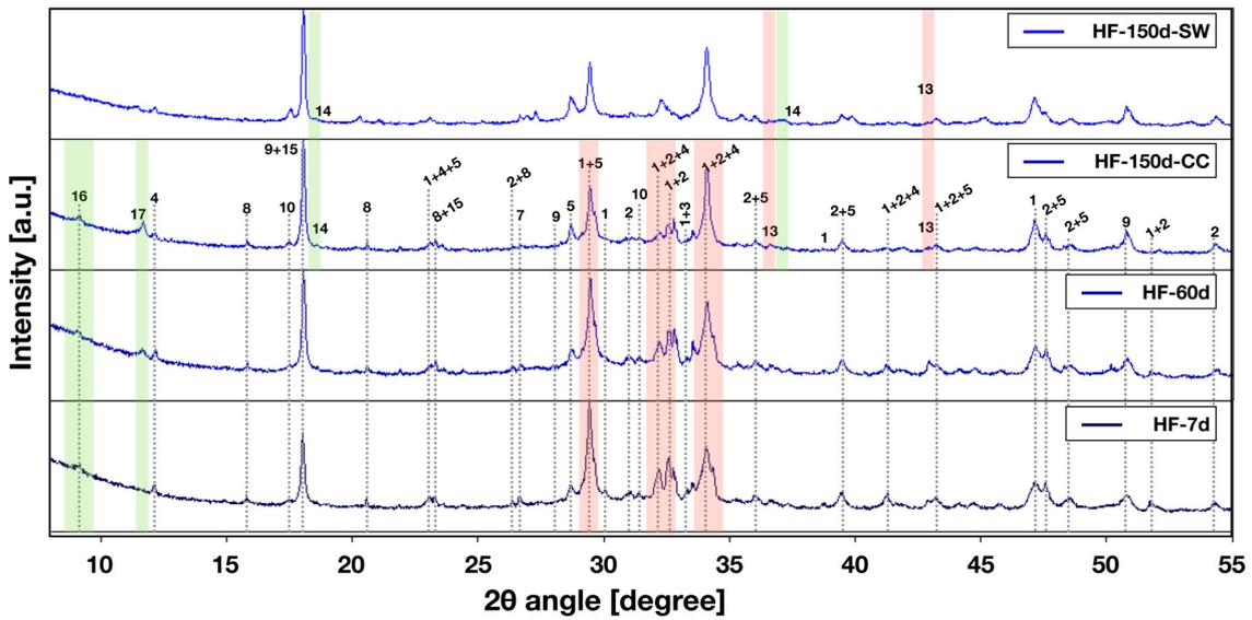
FIGURE 6. XRD diffractograms of HF at 7, 28, 60, and (for the samples exposed to two different curing environments only) 150 curing days, where annotations indicate: (1)  $C_3S$ ; (2)  $\beta-C_2S$ ; (3)  $C_3A$ ; (4)  $C_4AF$ ; (5) calcite; (7) quartz; (8)  $\gamma-C_2S$ ; (9) portlandite; (10) gehlenite; (13) periclase; (14) brucite; (15) mayenite; (16) AFt; and (17) AFm- $CO_3$ .
