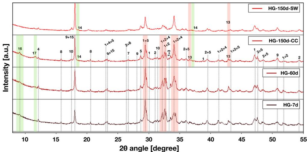
FIGURE 5. XRD diffractograms of HG at 7, 28, 60, and (for the samples exposed to two different curing environments only) 150 curing days, where annotations indicate: (1)  $C_3S$ ; (2)  $\beta$ - $C_2S$ ; (3)  $C_3A$ ; (4)  $C_4AF$ ; (5) calcite; (7) quartz; (8)  $\gamma$ - $C_2S$ ; (9) portlandite; (10) gehlenite; (13) periclase; (14) brucite; (15) mayenite; (16) AFt; and (17) AFm- $CO_3$ .
