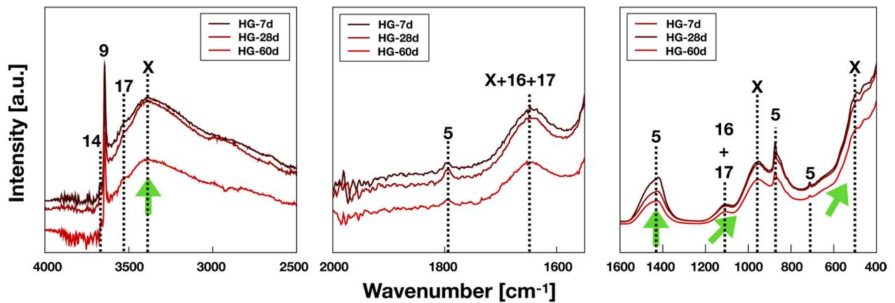
FIGURE 7. ATR-FTIR spectra of HG at 7, 28, and 60 curing days, where annotations indicate: (X) C-S-H gel; (5) calcite; (9) portlandite; (14) brucite; (16) AFt; and (17) AFm.
