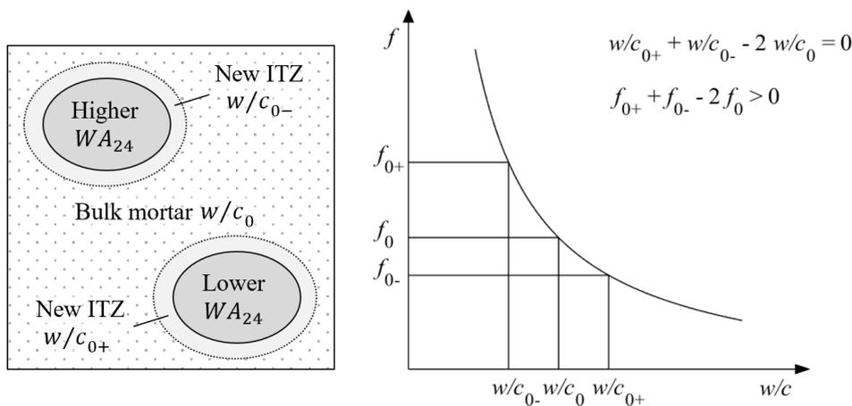
**FIGURE 8.** Hypothesis for a positive effect of local water/cement ratio variations in the new interfacial transition zone (ITZ) on the macroscopic compressive strength of concrete.
