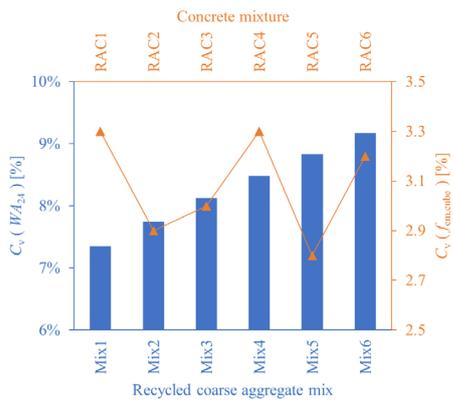
FIGURE 6. Comparison between variation coefficient of water absorption of recycled coarse aggregate mix and variation coefficient of compressive strength of concrete.
