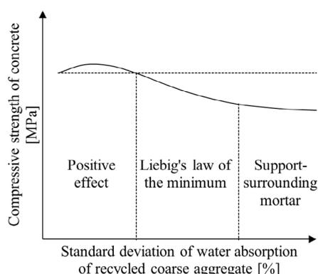
FIGURE 9. Hypothesis for the compressive strength of concrete as a function of standard deviation of water absorption of recycled coarse aggregate (when the mean value is constant).
