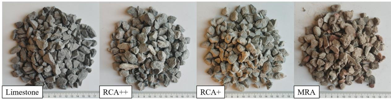
FIGURE 1. Photos of coarse aggregates.
