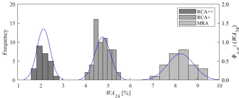
FIGURE 3. Water absorption distribution of recycled coarse aggregates.
