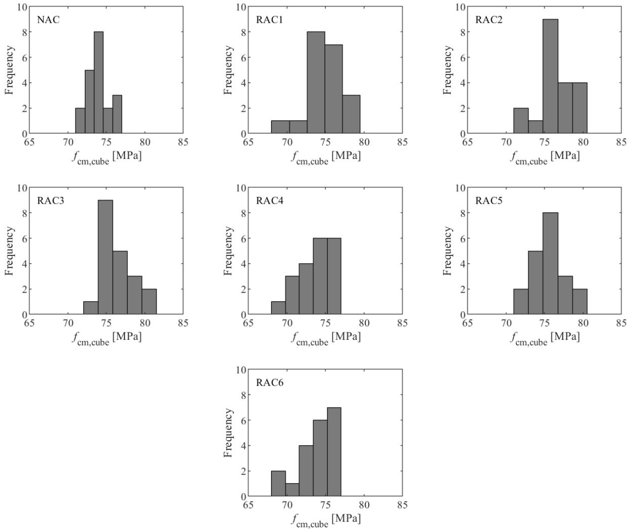
FIGURE 5. Cube compressive strength distribution of concrete mixtures.
