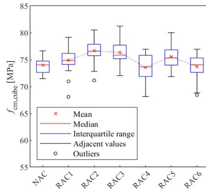
FIGURE 7. Cube compressive strength evolution of concrete mixtures.
