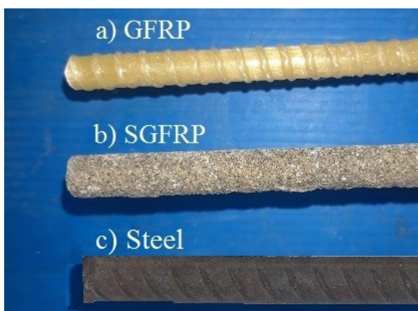
FIGURE 4. Composite rebars (GFRPS, GFRP) and steel rebar.
