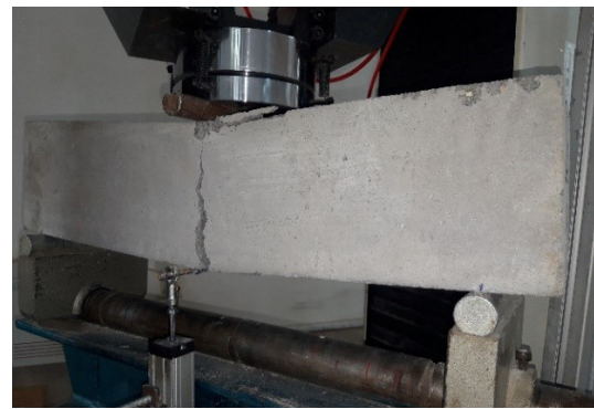
FIGURE 16. Beam specimen under three-point bending test.
