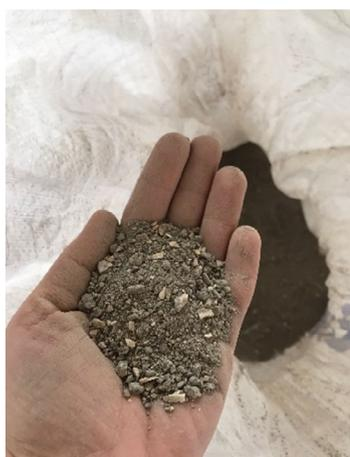
FIGURE 1. Recycled Asphalt Pavement (RAP).
