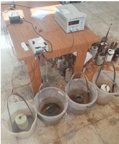
FIGURE 2. Accelerated corrosion test setup.
