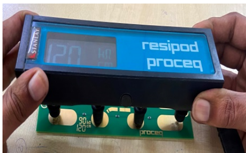
FIGURE 8. Resistivity meter setup and sample testing process.
