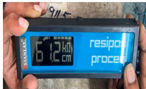
FIGURE 8. Resistivity meter setup and sample testing process.
