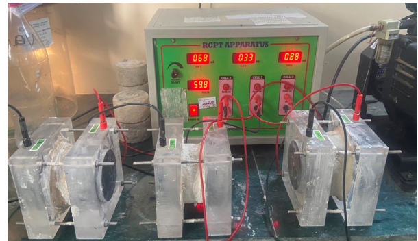
FIGURE 10. Standard configuration of RCPT unit (ASTM C1202).
