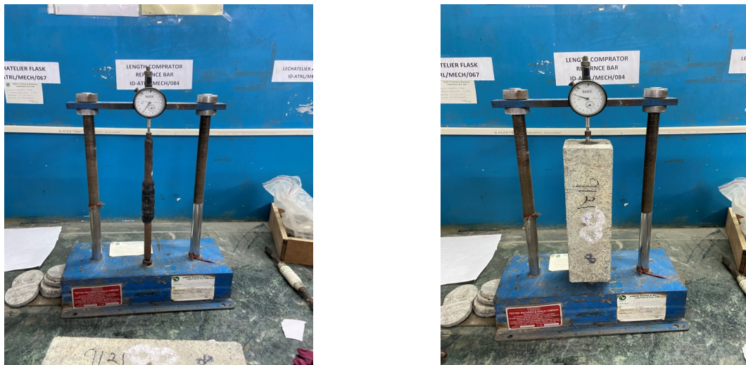
FIGURE 6. Drying shrinkage apparatus and sample testing process.
