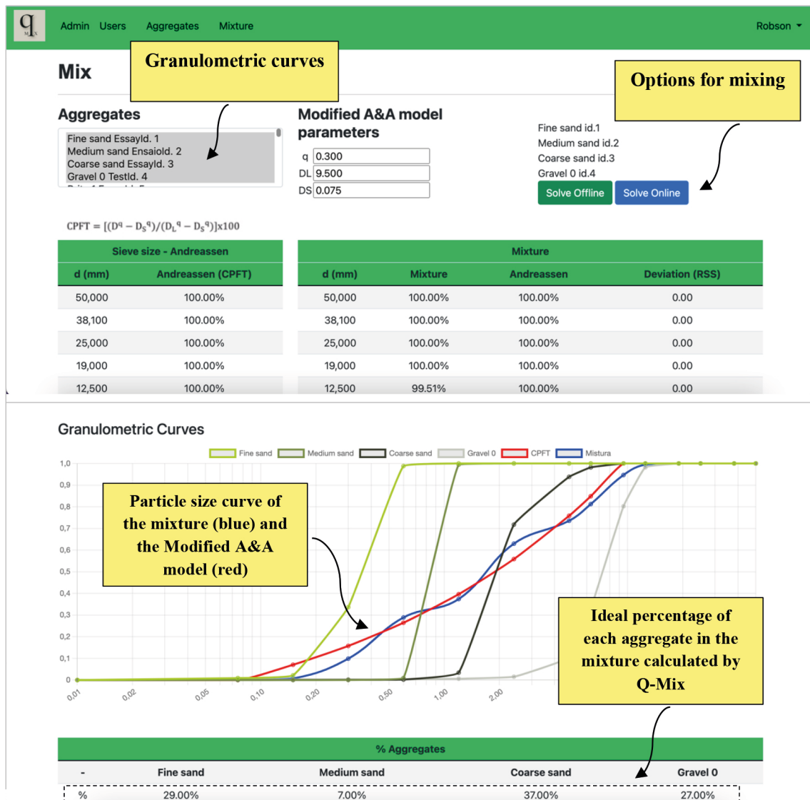
FIGURE 3. Example of packing calculation for three chemical a content of aggregates in Q-Mix.
