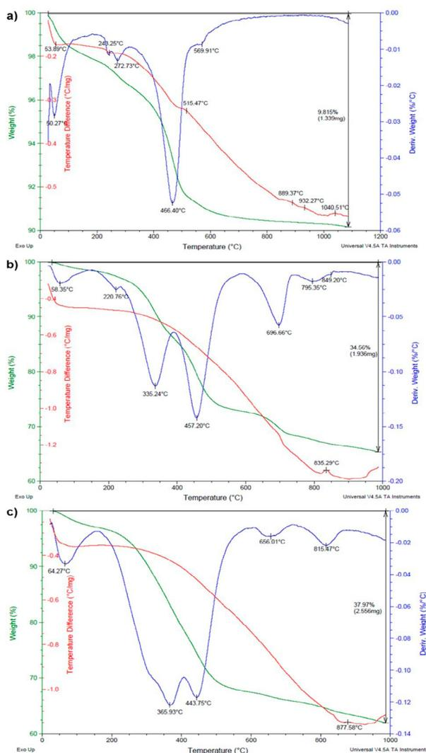
FIGURE 3. DTA-TG and DTG curves: a) Clay, b) SBC, and c) SBE.
