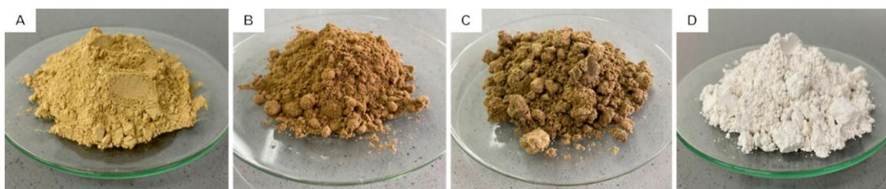
FIGURE 1. a) Clay (C), b) Spent bleaching earth (SBE), c) Spent bleaching earth with lime (SBC), and d) glass sediment (GS).
