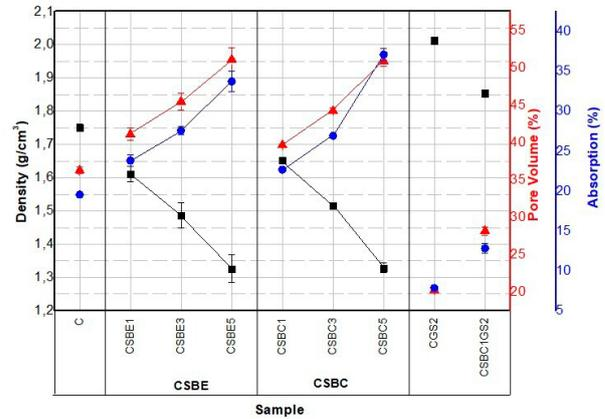
FIGURE 5. Apparent density (black), porosity (red) and water absorption (blue) results.
