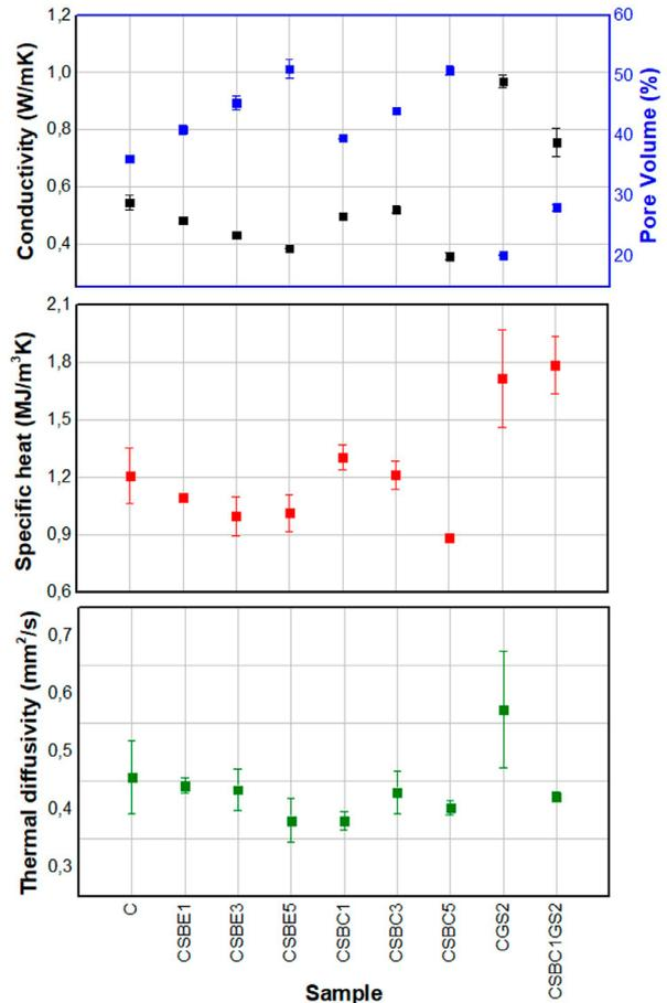
FIGURE 7. Thermal properties of the products.
