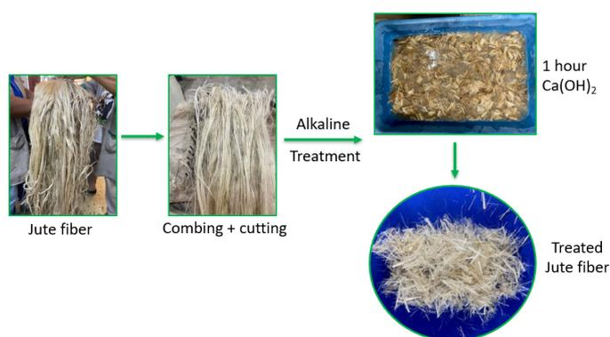
FIGURE 1. Processing and alkaline treatment of jute fibers.
