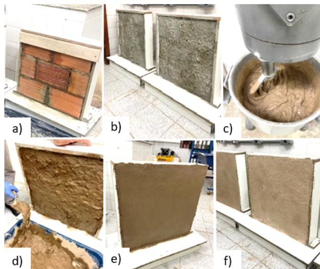
FIGURE 4. Production of wall samples. a) construction of hollow brick masonry, b) roughcasting, c) preparation of rendering mortar, d) application of rendering mortar, e) finishing and smooth surface, and f) curing.
