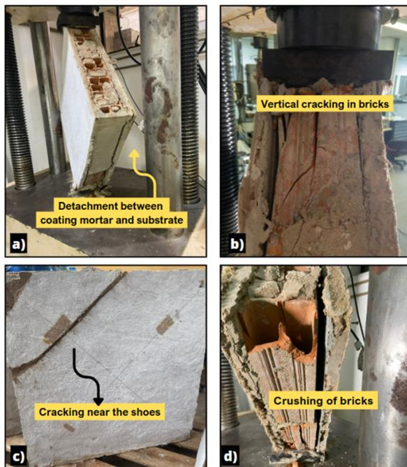
FIGURE 15. Failure modes of the test specimens. a) detachment of the plaster, b) cracks in the bricks, c) cracks in the masonry in contact with the footing, d) crushing of the brick.
