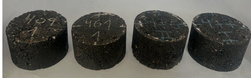
FIGURE 2. (Left) Reference mix-HMA-R (Left-center) Modified mix-WMA-1(Right-center) Modified mix-WMA-2(Right) Modified mix-WMA-3.
