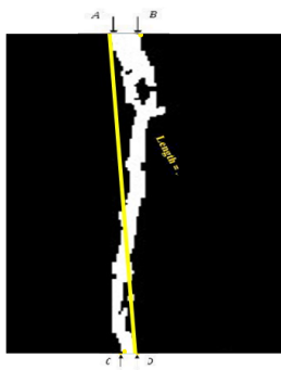
Figure 12. Measurement of the crack length.
