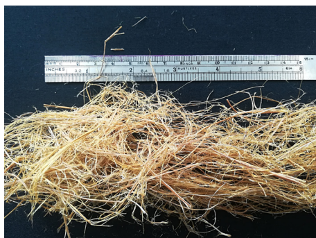
FIGURE 11. Guadua fibers obtained using the proposed extraction methodology.
