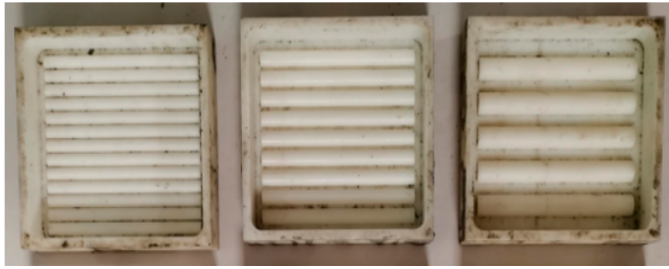
FIGURE 5. Concrete block test molds.
