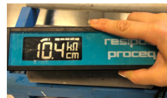
FIGURE 4. Measurement of electrical resistivity on a cylindrical specimen.
