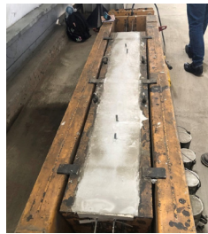
FIGURE 3. Pre-stressed concrete sleeper for industrial scale validation.
