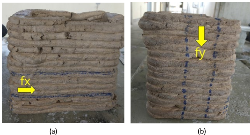
Figure 8. Cutting the blocks to obtain the test pieces (a) representation of the cut in the fx direction and (b) representation of the cut in the fy direction.
