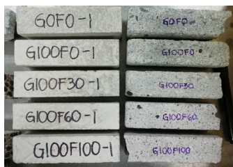
FIGURE 11. Samples without paste improvement: Control samples without PSA (A) and damages to the PSA test (B).
