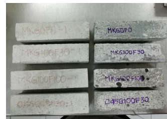
FIGURE 12. Improved cement paste: Control samples without PSA (A), and damage due to the PSA test (B).
