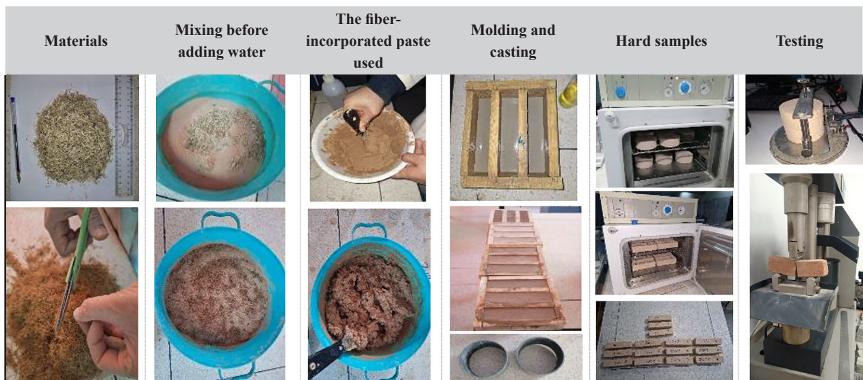
FIGURE 10. The steps involved in preparing biobased adobes.
