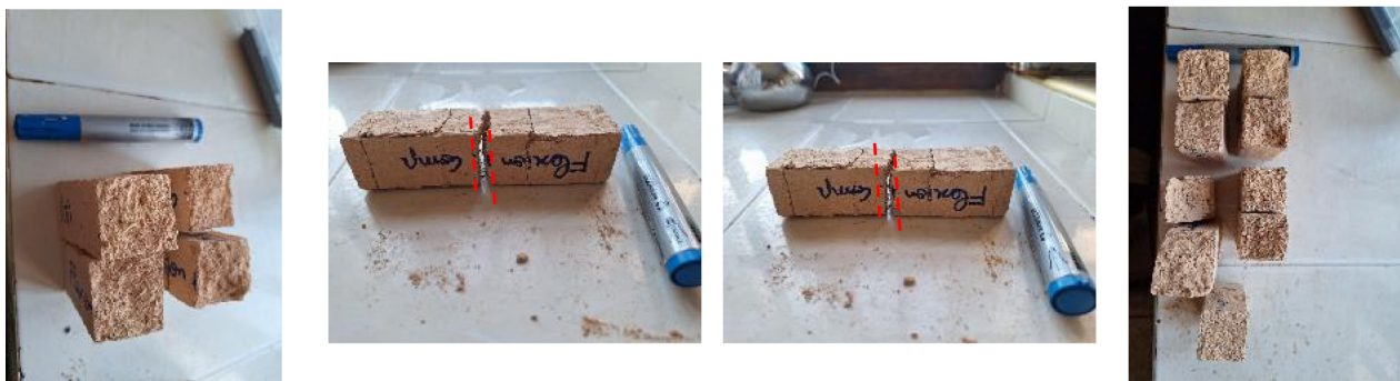
FIGURE 15. Observation of sample break-up surface after destructive testing.
